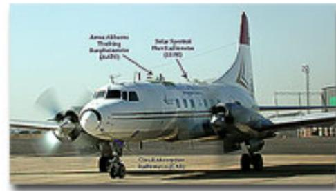
The CAR instrument is housed in the nose cone of the CV-580 aircraft. In this photo, CAR's stainless steel sliding door is in the closed position, protecting the scan mirror and optics assembly from dust and other foreign objects during takeoff and landing.
