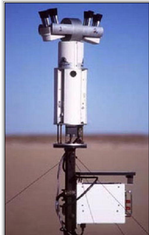
The PARABOLA III scanning radiometer. Shown are the four sensor heads (each with four spectrally-filtered radiometers), a reflectance standard, power supply, Zip drive housing, and guy-wired stand.
