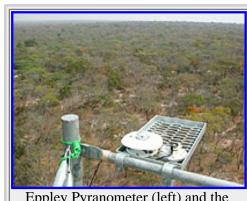
Eppley Pyranometer (left) and the Skye SKE 510 (right) together on a platform on the Mongu Tower.
