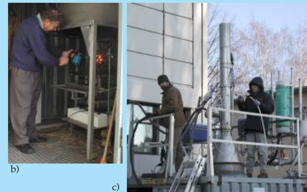
Fig. 2. a) Diagram of burning facility at MPI; b) technician igniting center of branch sample stacked on burn table positioned at 10°; and c) sampling equipment deployed on roof of facility.
