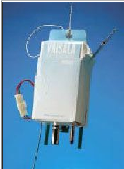
Standard Vaisala radiosonde instrument package RS80, which hangs under a balloon.
