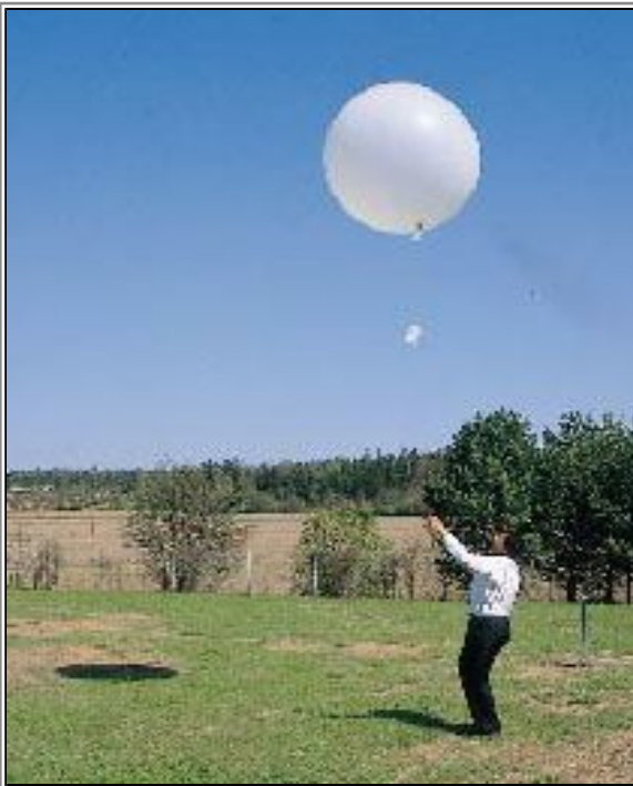
The radiosonde is launched using a balloon.
