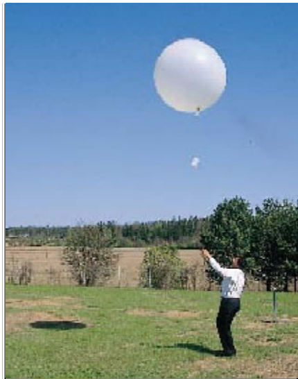
The radiosonde is launched using a balloon.
