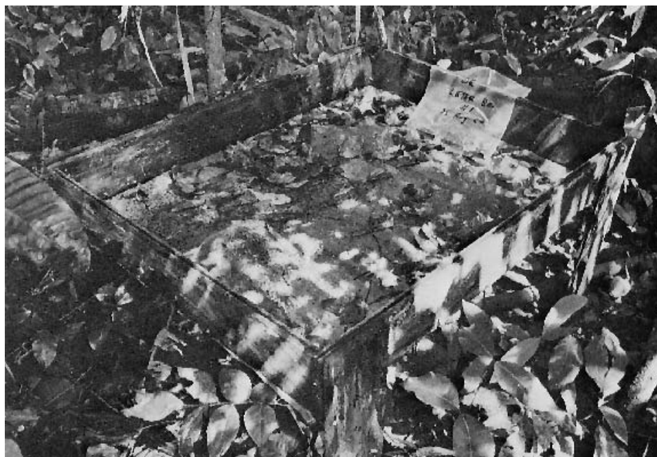
Figure 5. A litter collection box in the forest at the Darien study site, Panama. (The box is approximately one meter square and is held 20 cm above the forest floor by wooden legs. Photograph by F.B. Golley, University of Georgia, and co-authors. Reproduced by kind permission of F.B. Golley and the University of Georgia Press).
