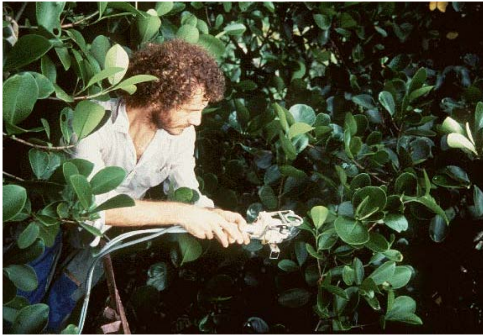
Figure 3. Use of a portable photosynthesis system for leaf gas exchange measurements at the Barro Colorado tropical forest site, Panama. (Gerhard Zotz, a German doctoral student, is using a clampon leaf chamber and infra-red gas analyzer [Heinz Walz, Effettrich, Germany] on leaves of Clusia uvitana . Photograph taken around 1995 by Marcos Guerra, STRI).
