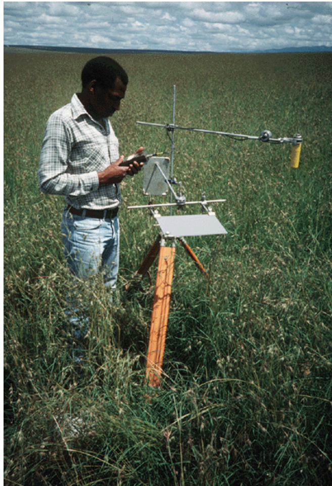
Figure 1. Canopy reflectance measurement within the Nairobi grassland site, Kenya. (Prof. Jenesiso Kinyamario, University of Nairobi, is using a red/near-infrared spectral ratio meter. Photograph taken May 1986 by Dr. J.M.O. Scurlock, ORNL).
