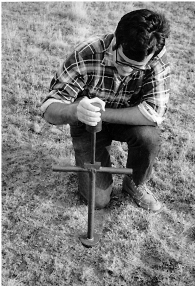
Figure 9. Measurement of below-ground biomass at the CPER/Pawnee grassland site, Colorado, USA. (Dale Bartos, Colorado State University, is using a root core sampler fitted with a slide-hammer. Photograph taken 1970-1972 by Dan Uresk, Colorado State University).
