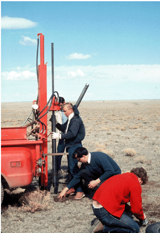
Figure 10. Soil coring apparatus mounted on the back of a pick-up truck at the CPER/Pawnee grassland site, Colorado, USA. (John Leetham, Research Technician, Colorado State University, is operating the soil corer; other persons not identified. Photograph taken April/May 1971 by Larry Nell, Colorado State University).
