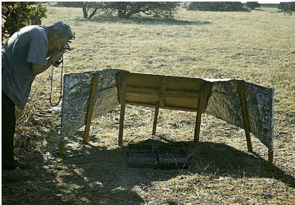
Figure 4. Experiment to study the effect of UV-b solar radiation on litter decomposition at the Badkhyz grassland site, Turkmenistan. (Prof. Leonid Rodin, Komarov Botanical Institute, Leningrad, is photographing litter samples under a shade screen. Experiments at Badkhyz and elsewhere demonstrated considerable influence of solar radiation on decomposition rate. (Photograph taken October 1978 by Dr. R. Zlotin, Indiana University, Bloomington, IN, USA).
