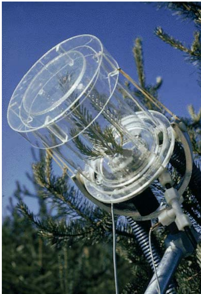
Figure 10. Temperature-controlled shoot cuvette for continuous measurement of gas exchange in young Pinus sylvestris at the Jdraas study site, Sweden. (Cooling air passes between the double walls of the chamber, and air from the center of the cuvette is circulated to an infra-red gas analyzer for analysis of CO 2 assimilation and respiration. Photograph taken summer 1975 by Dr. S. Linder, Swedish University of Agricultural Sciences, Uppsala).
