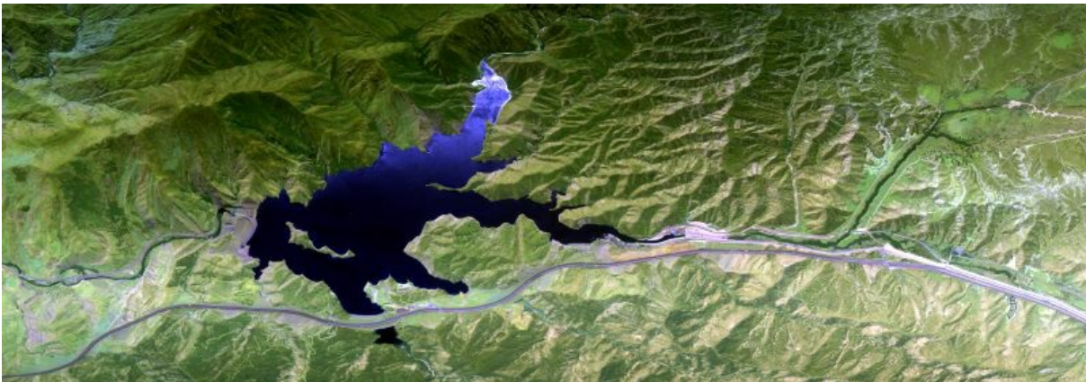
Figure 1. RGB composite image from data collected over Pyramid Lake, California, U.S. on 2009-07-24. Image derived from bands 12, 10, 9 spanning visible to near-infrared wavelengths. Source: MASTERL1B_0901100_05_20090724_2125_2126_V01.hdf
