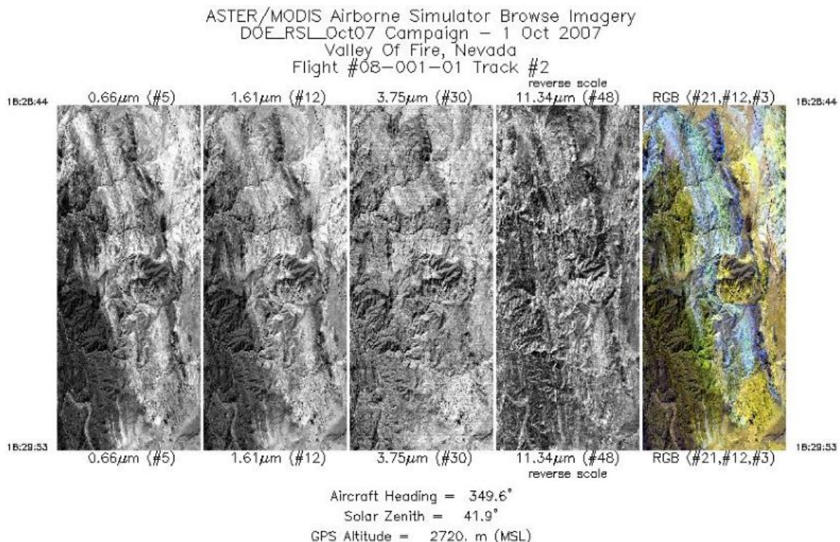
Figure 1. Single-band images and a RGB composite image from flight track 2 as acquired on 01 October 2007 over Valley of Fire, west of Lake Mead, Nevada, California, U.S. Source: MASTERL1B_0800101_02_20071001_1828_1829_V02.jpg
