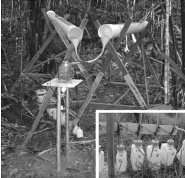
Figure 3: Sequential sampler design: Composite of two through collectors, a tipping bucket and 10 sampling bottles. The detail image in the lower right image corner shows individual sampling bottles and the connection tubing.
