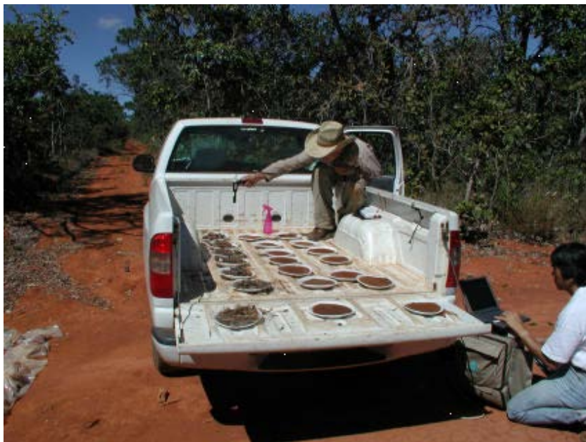
Figure 4. ASD measurements being taken of soil and litter samples.
