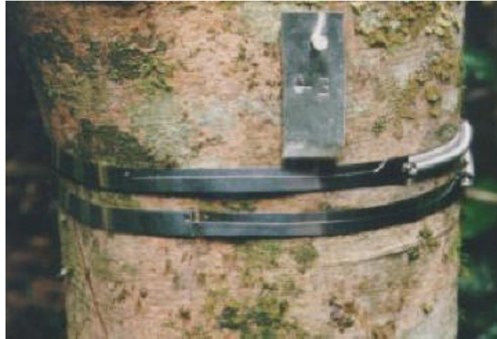
Figure 1. Dendrometer bands wrap like a belt around a tree at breast height. A spring secures the ends and two measuring points are punched where the band overlaps. An initial diameter at breast height is recorded for each tree. As the tree grows, the spring stretches, and the measuring points are pulled apart. By measuring this increasing distance between points, we can accurately determine the increase in the tree's diameter. Most trees have only one dendrometer, but this tree was being used to test different dendrometer styles.
