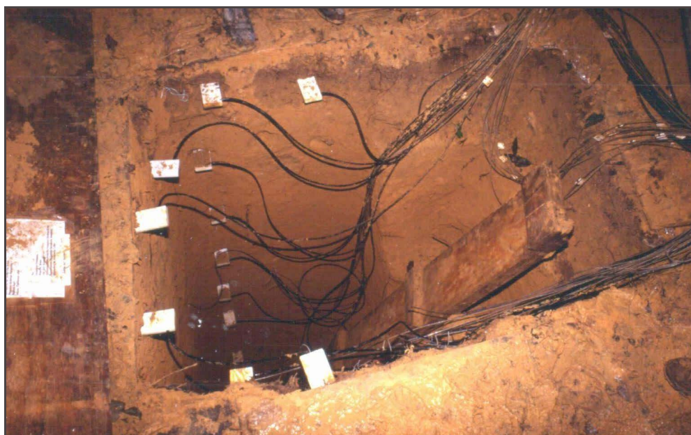
Figure 1. Soil moisture measurements were made in 10 m deep vertical pit (1 x 1 m 2 ) approximately 20 m from the micrometeorological tower sites in undisturbed forest patches. Reflectometers were inserted horizontally into shaft walls at 0.15, 0.30, 0.60, 1, 2, 3, 4, 6, 8, and 10 meters beneath the surface.
