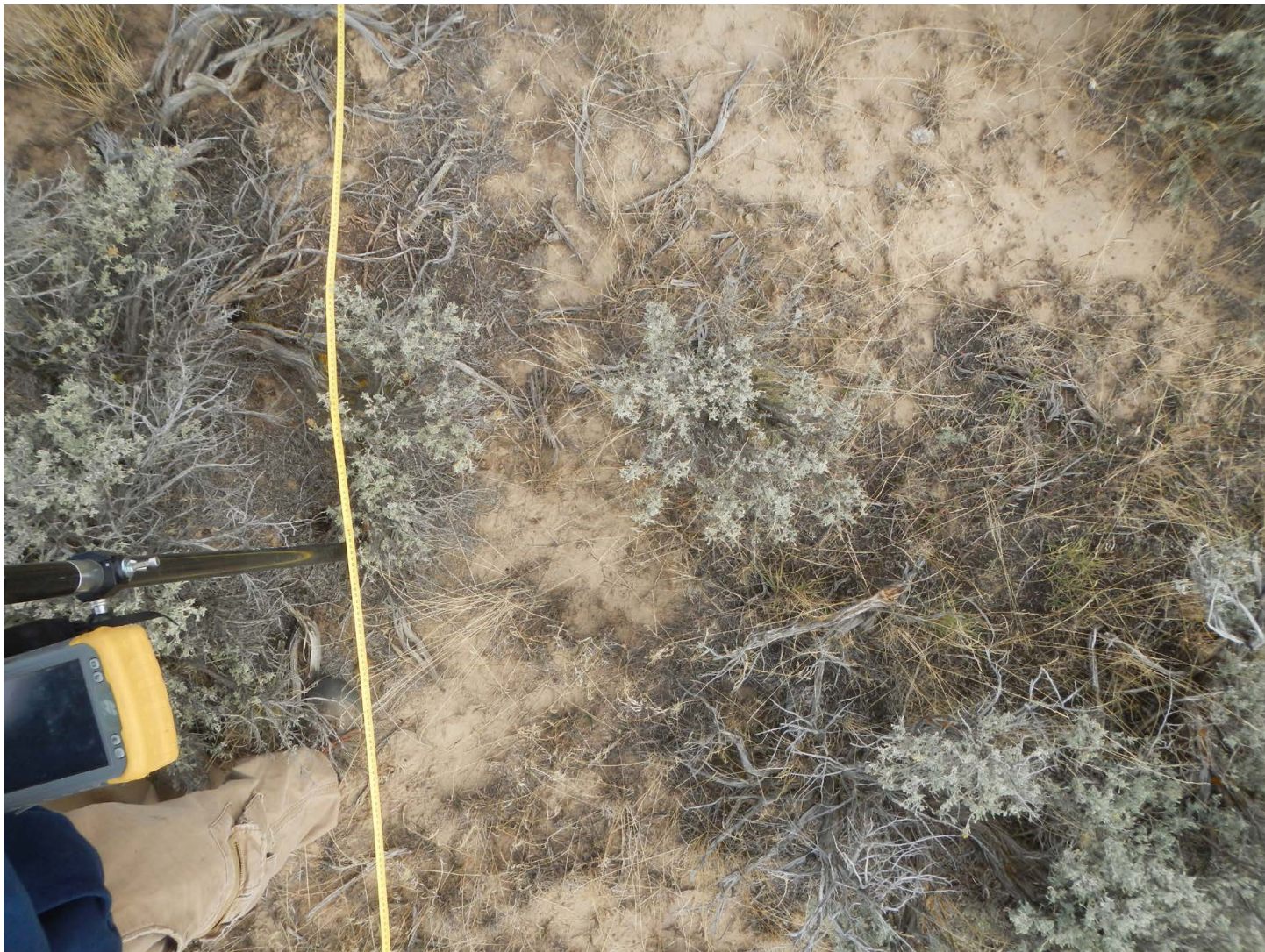
Figure 1. Typical plot photo for ground cover estimates and location of LAI measurements. A range pole with GPS and a camera boom was positioned at 2-meter intervals along plot transects. This photo is from the Hollister, Sagebrush01 plot, and the Sagebrush01_5_4 sampling point.
