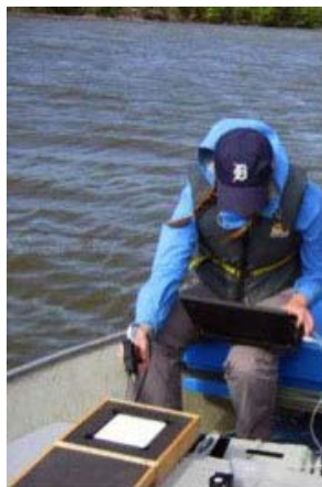
Figure 6. Spectrometer being used in the field to collect a white reference measurement.
