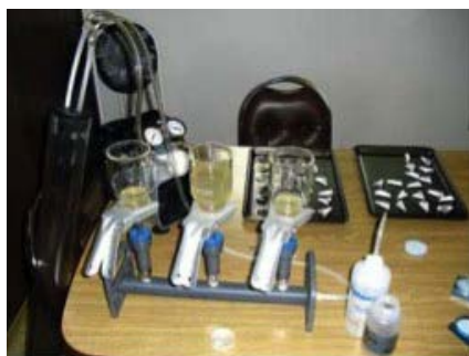
Figure 5. Vacuum filtration system used to quantify suspended sediment concentration in water samples.
