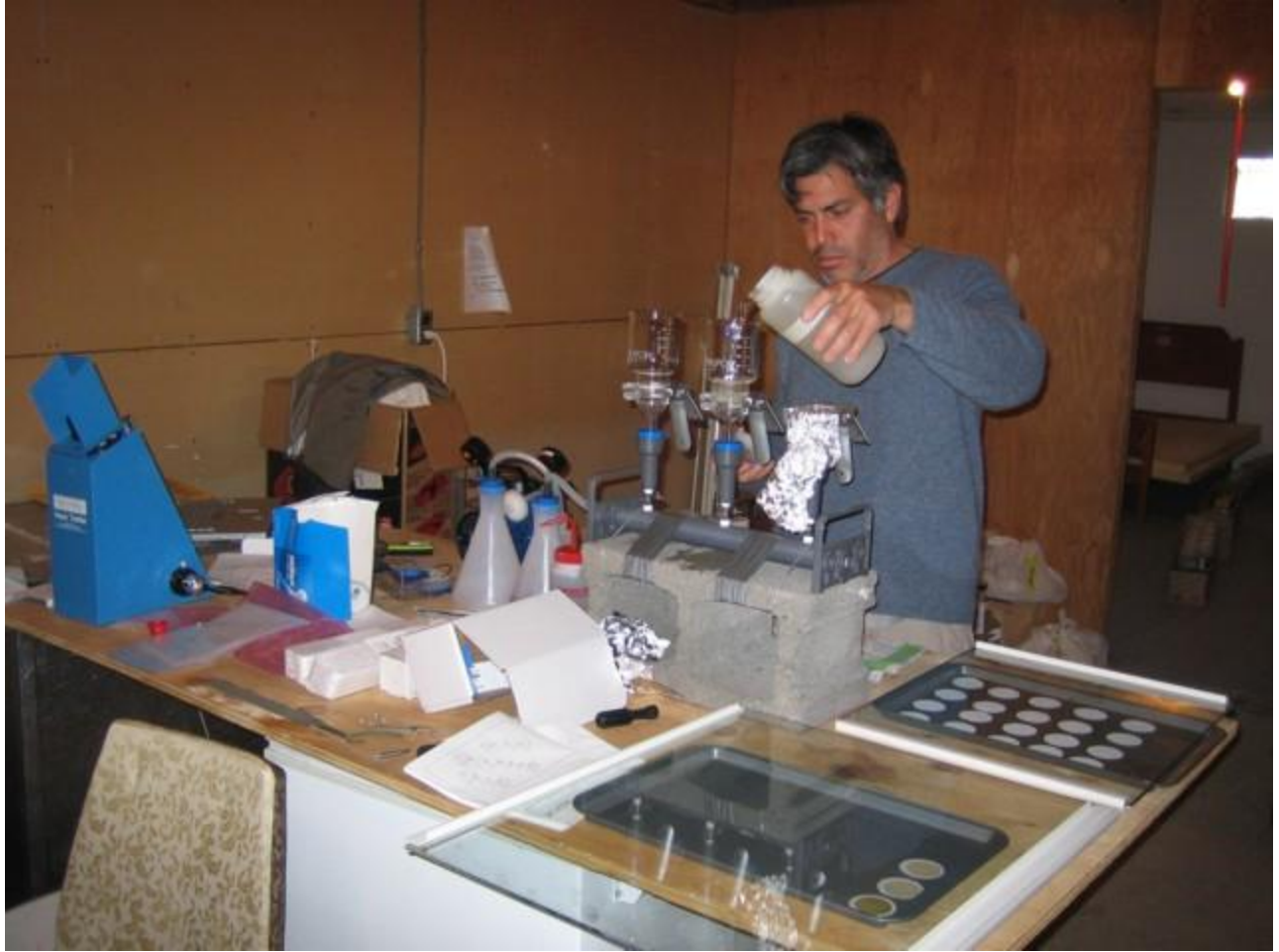
Figure 6. Suspended solids filtration equipment.
