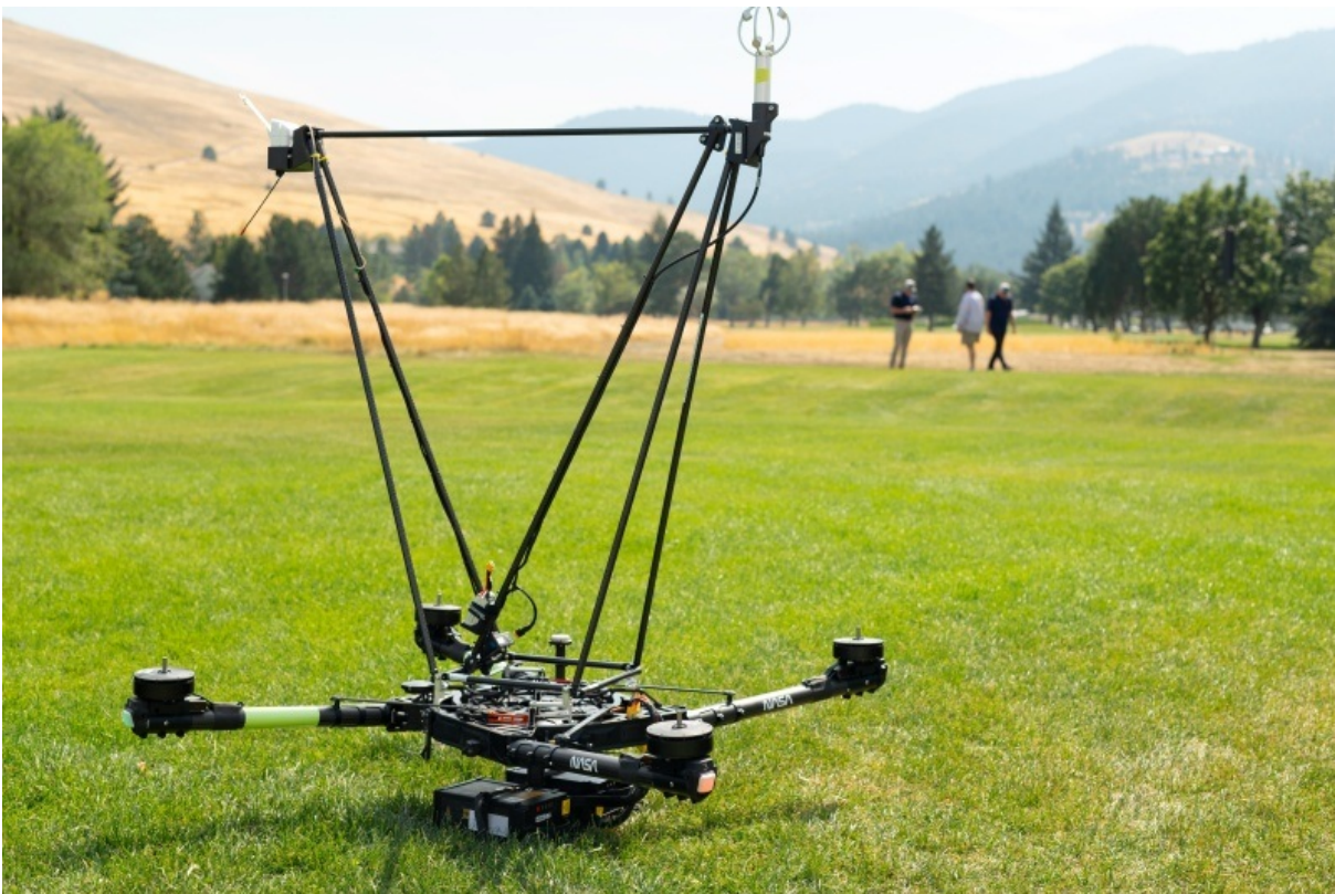
Figure 1. The NASA Alta X quadcopter sits in a field in Missoula, Montana, outfitted with a structure engineered at Langley Research Center to carry a radiosonde (top left) and an anemometer (top right) into the air. The UAS and its payload were part of the August 2024 FireSense campaign, which examined the applicability of using controllable, repeatable airborne measurements to more accurately predict fire and smoke behavior. Image Credit: NASA ARC/Milan Loiacono.
