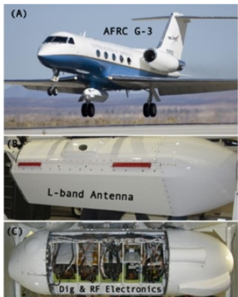
Figure 2. UAVSAR is flown on a Gulfstream-III aircraft, mounted in a pod hung below the fuselage.
