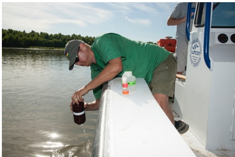
Figure 1. Collection of surface water samples in the Atchafalaya River for total suspended solids (TSS) analysis.
