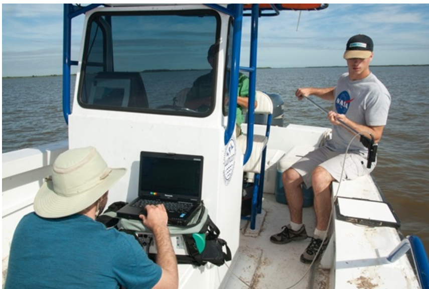
Figure 1. Collecting in situ spectral reflectance data with the Analytical Spectral Devices (ASD) FieldSpec 3 on the Atchafalaya River. Radiance measurements from the white reference panel are used to normalize radiance measurements from the water surface to calculate water-leaving reflectances, which were then used to derive remote sensing reflectances.
