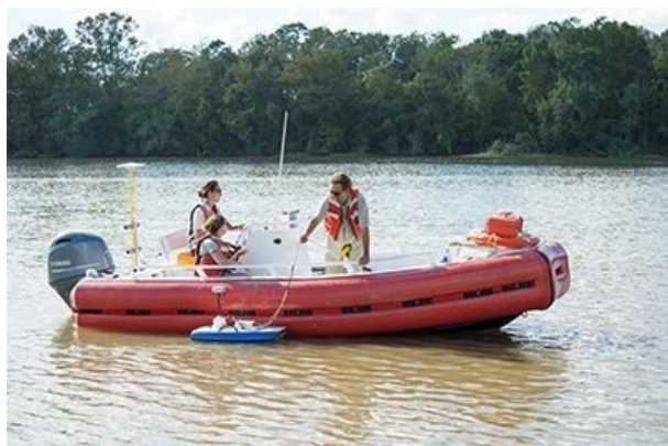
Figure 1. Measurement of river discharge across channels. The acoustic doppler current profiler (ADCP) was mounted on a hydro board, which was allowed to drift alongside the boat while maintaining a transect perpendicular to flow. The impact from the boat was limited by slowly crabbing across each channel, allowing the ADCP to remain on the upstream side of the boat.
