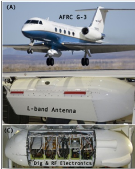
Figure 2. (A) UAVSAR is flown on a Gulfstream-III aircraft, mounted in a pod hung below the fuselage. The antenna is left-side looking. The pod contains (B) the antenna and (C) the digital and RF electronics. The recording media are housed within the fuselage.
