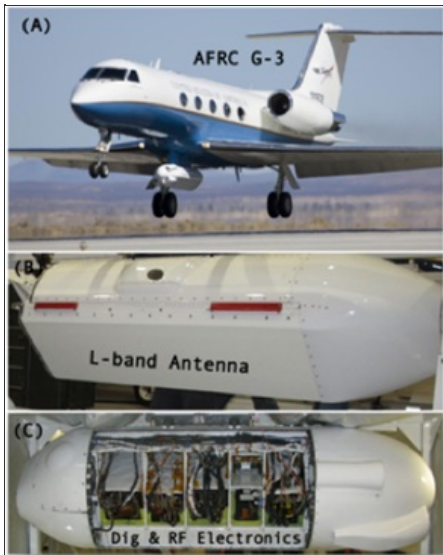
Figure 2. (A) UAVSAR is flown on a G-3 aircraft, mounted in a pod hung below the fuselage. The antenna is left-side looking. The pod contains (B) the antenna (left-side looking) and (C) the digital and RF electronics. The recording media are housed within the fuselage.
