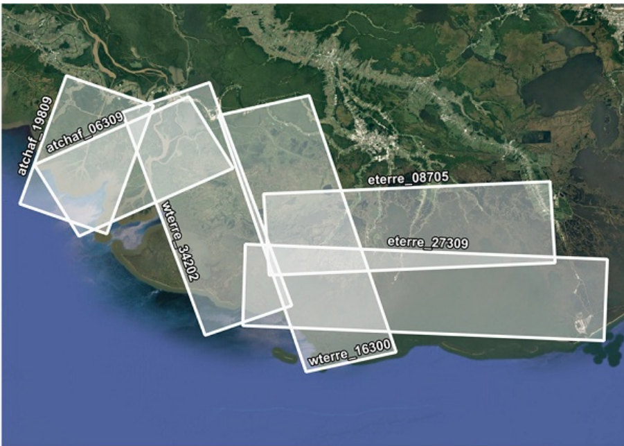
Figure 4. Spatial coverage of each UAVSAR flight line acquired during the 2021 Delta-X campaign. Shown are the Atchafalaya and Terrebonne Basins along the southern coast of Louisiana, USA.
