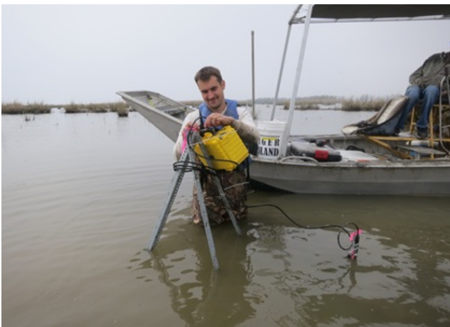
Figure 1. Installation of turbidity sensor in Mike Island study area of the Wax Lake Delta in coastal Louisiana.
