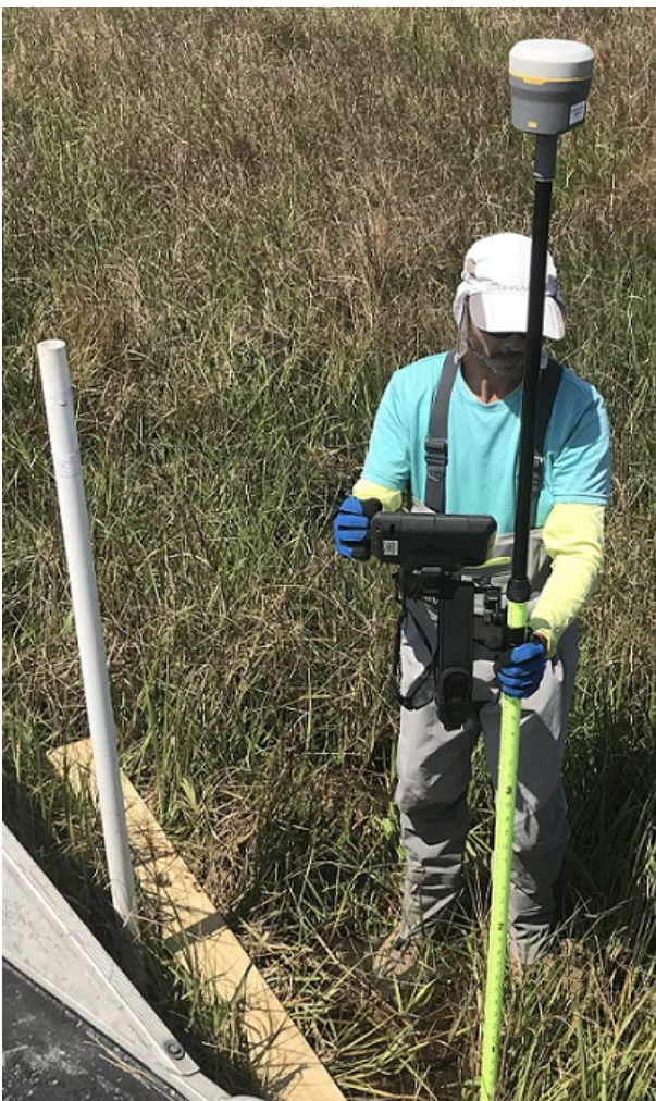
Figure 1. GPS elevation measurements being taken in the field during the Delta-X Spring Campaign in March and April 2021.
