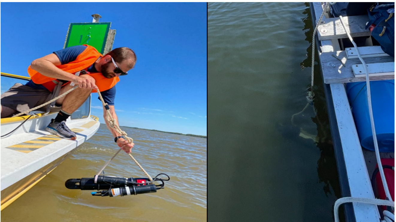
Figure 1. LISST-200X being deployed by hand off the side of the boat (left), and position of the deployed LISST-200X for the surface measurement (right).
