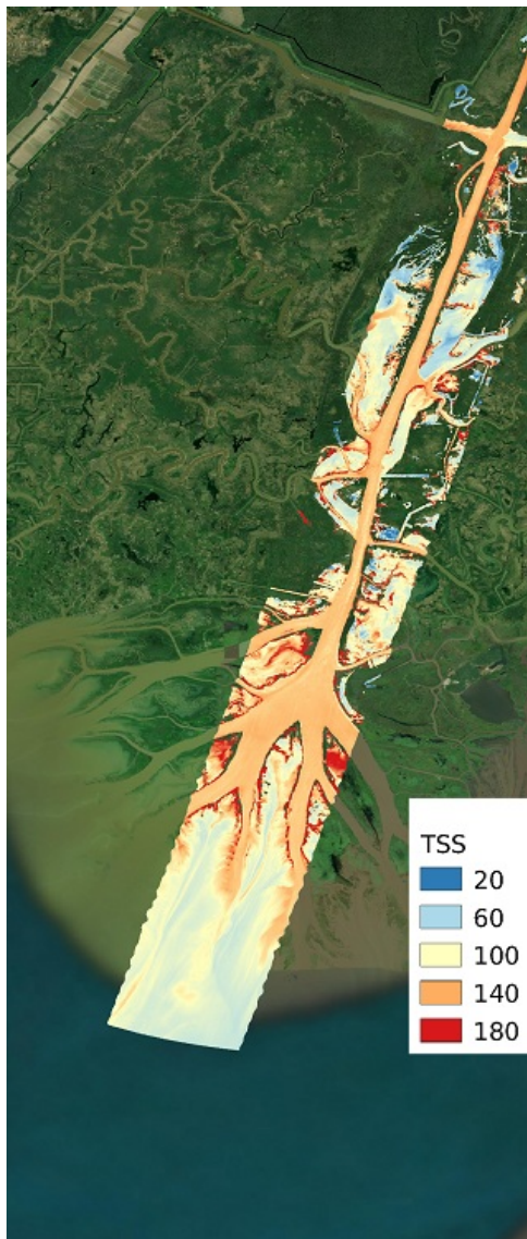
Figure 1. Map of total suspended solids (TSS) in the Wax Lake Delta, Terrebonne basin of the Mississippi River Delta of coastal Louisiana. TSS was estimated from AVIRIS-NG imagery using a regression model derived from in-situ measurements of surface reflectance and TSS.
