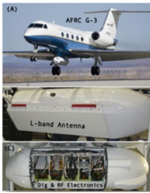
Figure 2. UAVSAR is flown on a Gulfstream-III aircraft, mounted in a pod hung below the fuselage.
