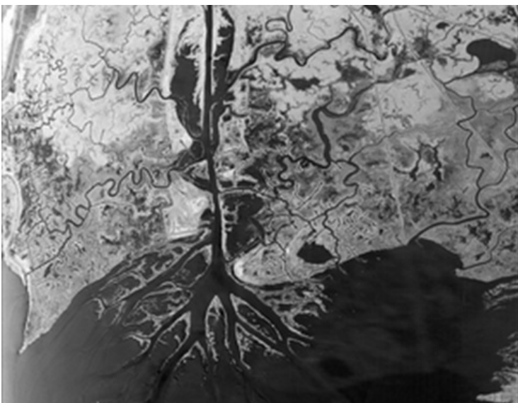
Figure 1. A single image product from the UAVSAR SLC stack atchaf_19809_02 collected on 27 March 2021, over the Atchafalaya Basin, Louisiana. The image shows the amplitude of the HH-polarization SLC data in radar coordinates.
