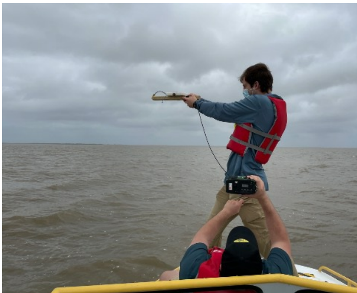
Figure 1: Collection of water-leaving radiance measurement using the Portable SpectroRadiometer (PSR).
