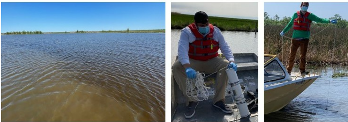
Figure 1: Types of waters being sampled in this study region (left), van Dorn sampler being used to collect surface samples (middle), and deployment of van Dorn sampler (right).
