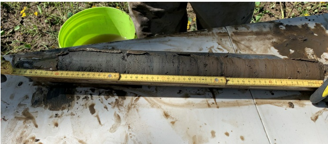
Figure 1. Typical soil core from herbaceous wetland collected during March 2021 in coastal Louisiana. This image shows the top 50 cm of soil collected using a Russian corer.
