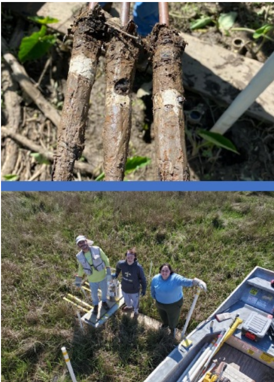
Figure 1. Top image: Cryocores showing sediment deposited on top of feldspar marker horizon; Bottom image: Feldspar station set up.
