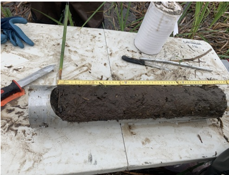
Figure 1. Root biomass sample (top 50 cm of soils) collected using a gouge soil auger.
