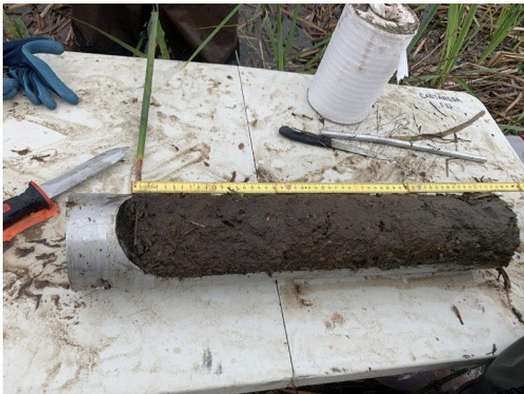
Figure 1. Root biomass sample (top 50 cm of soils) collected using a gouge soil auger.
