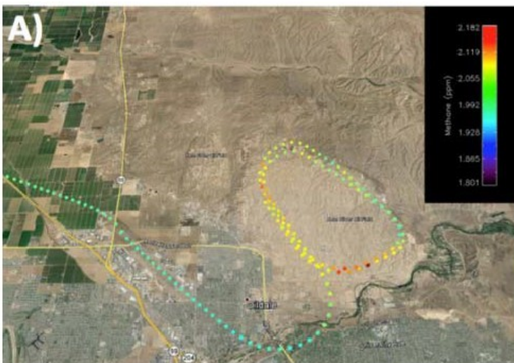
Figure 1. Methane concentrations from the Alpha Jet over Kern River oil field and environs in California on 10 June 2014. Source: Krautwurst et al. (2016).
