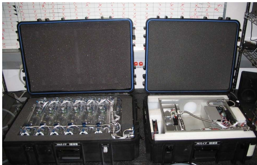
Figure 3. Flask sampling system for aircraft measurements. Left: Programmable Flash Package (PFP) containing 12 flasks. Right: Programmable Compressor Package (PCP) containing pumps for pressurizing the flasks. (Image courtesy: http://www.esrl.noaa.gov/gmd/ccgg/aircraft/sampling.html )
