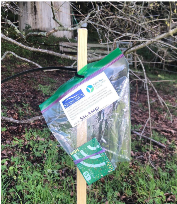
Figure 2. An AudioMoth automated recorder placed within a plastic ziplock bag.
