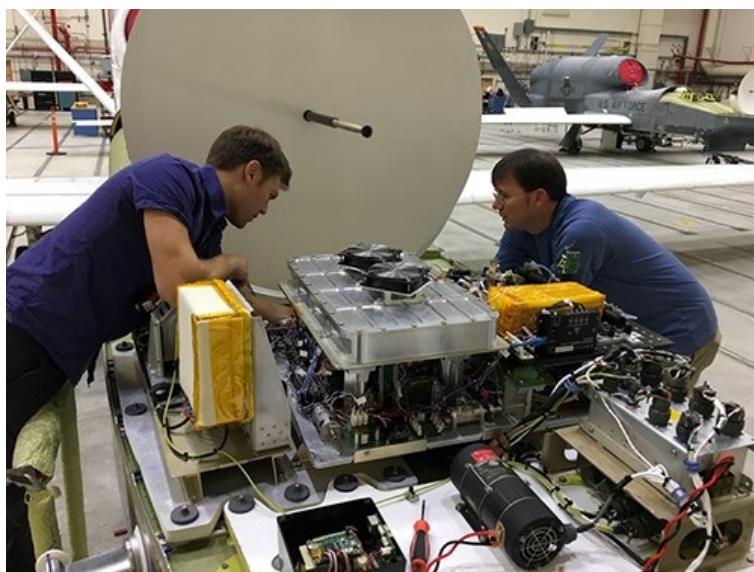
Figure 1. Photograph of the laser-induced fluorescence instrument described in Rollins et al. (2016) during development. Source: https://csl.noaa.gov/groups/csl6/instruments/so2/
