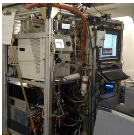
Figure 2. The HR-AMS instrument installed on the NASA DC-8 for the ATom-1 deployment.
