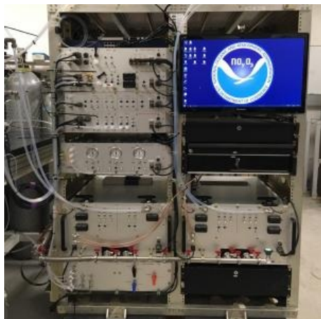
Figure 1. The NOAA NO y O 3 4-channel chemiluminescence (CL) instrument.
