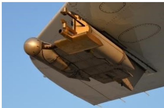
Figure 1: The CAPS instrument attached to the exterior of the NASA DC-8 aircraft.
