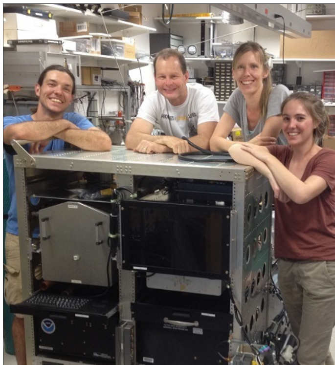
Figure 2. The aerosol microphysical properties (AMP) instrument package. Five instruments, two nucleation-mode aerosol size spectrometers (NMASS; Williamson et al., 2018), two ultra-high sensitivity aerosol spectrometers (UHSAS; Kupc et al., 2018), and a laser aerosol spectrometer (LAS) comprise the AMP package.
