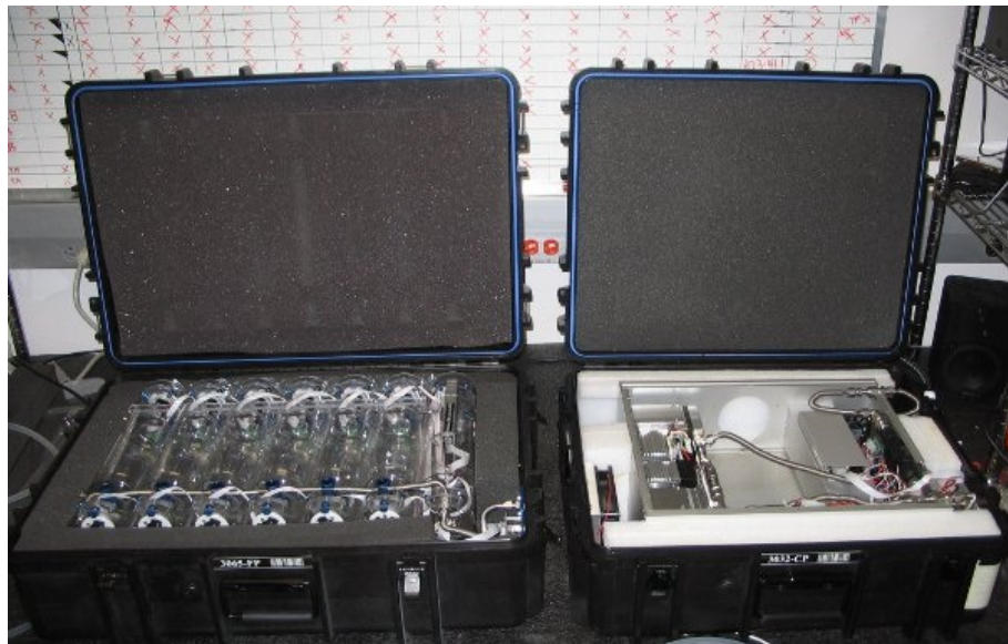
Figure 3. Flask sampling system for aircraft measurements. Left: Programmable Flask Package (PFP) containing 12 flasks. Right: Programmable Compressor Package (PCP) containing pumps for pressurizing the flasks. Source: NOAA Global Monitoring Laboratory
