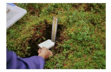
Try to minimize the amount of compaction and/or damage to the sample during extraction
