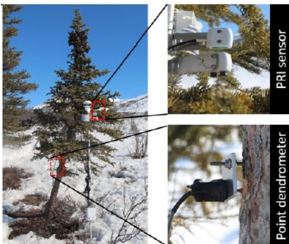
Figure 1. A white spruce tree is instrumented with a hemispherical and field-stop photochemical reflectance index (PRI) sensor and point dendrometer at a northern treeline site along the Dalton Highway, Brooks Range, Alaska. Source: Eitel et al., 2020
